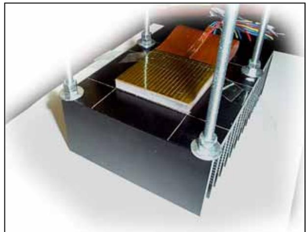
The sample is inserted in the flexible thin foil  $\Delta T$  sensor which consists of a series association of plated thermocouples indicating the temperature difference across the sample. The mV readout of the  $\Delta T$  sensor (about 2.2 mV for  $\approx 10^\circ\text{C}$ ) is translated in  $^\circ\text{C}$  and divided by the plate thickness in meter to give the temperature gradient in  $^\circ\text{C}/\text{m}$ .
