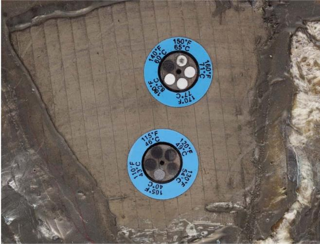
Fig. 10. Temperature has reached 65 °C on the top of a magnet during the measurements.
