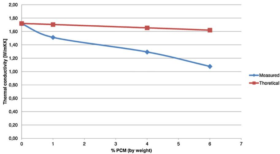
Fig. 3. Thermal conductivity of PCM concrete samples.
