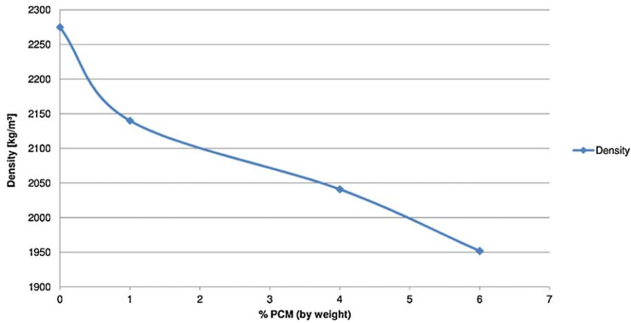
Fig. 2. Density of the PCM concrete samples.
