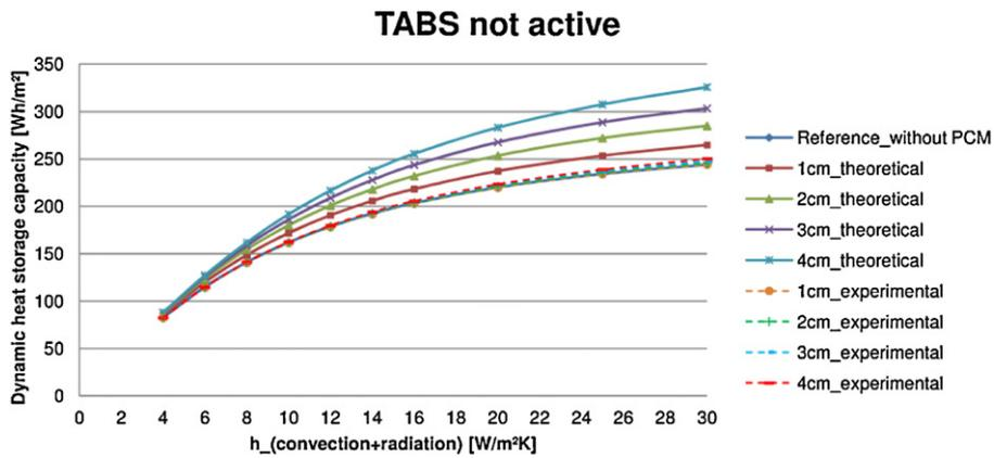
Fig. 12. Daily dynamic heat storage capacity of the deck with reference concrete and theoretically/experimentally determined 6 wt% PCM concrete.
