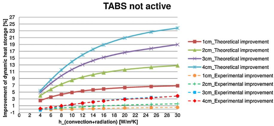
Fig. 11. Calculated improvement of the dynamic heat storage of deck with theoretically/experimentally determined 4 wt% PCM concrete with regard to the deck without PCM.
