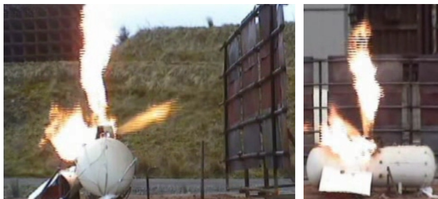
Fig. 6. Ignited release of propane from fittings.
