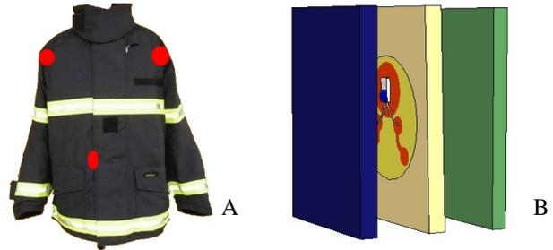
Figure 1: sensor integration in the firefighter jacket. A) Platinum sensors were located on the left and right shoulders and on the chest. B) The modified platinum probes were integrated on each side of the thermal insulation layer, between the comfort layer (green) and the external layer (blue).
