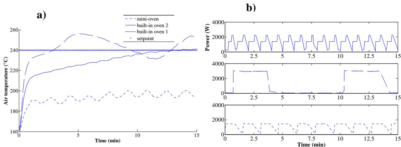
**Figure 2.** Cooking of three “cordons-bleu” in the three tested ovens (set point 240°C, free convection)
