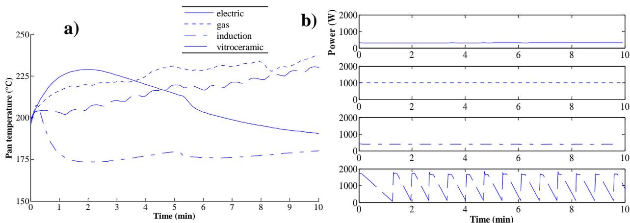
**Figure 1.** Cooking of three breaded poultry products for contact-heating devices (medium cooking power, pan #2)
