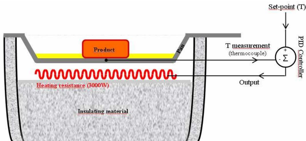
**Figure 3.** Schematic representation of original prototype developed for contact heating
