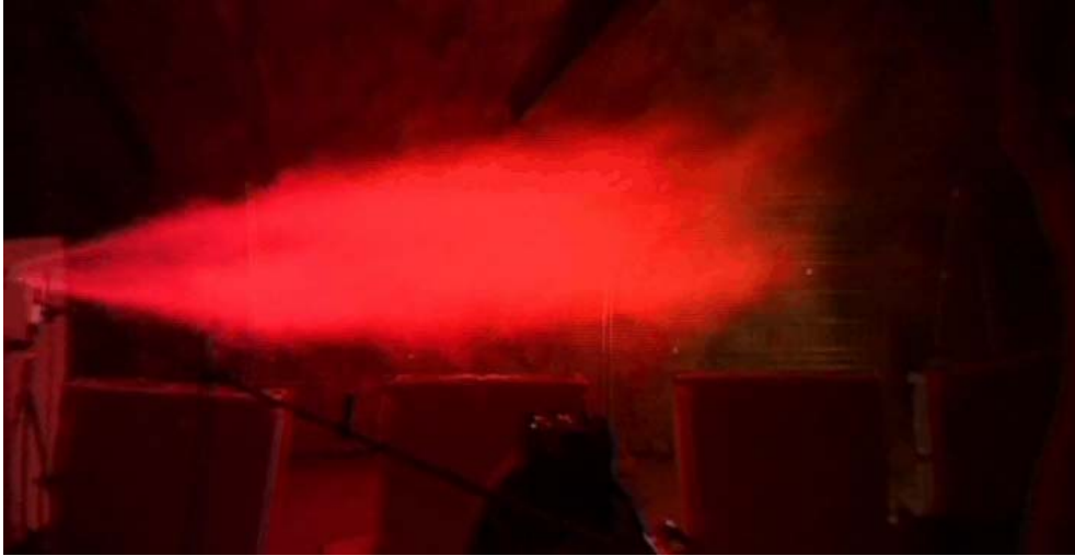
Figure 7 : view extracted from the video record of the blow down through a 3 mm orifice
