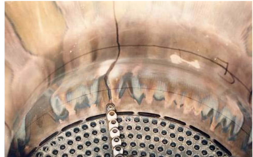
Blanching and cracking of SSME Chamber Liner
