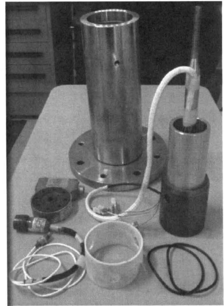
Figure 12. The Design and Parts for the Tungsten Piston Calorimeter
