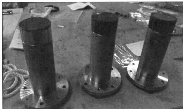
Figure 13. HY-80 witness rods ready for installation
