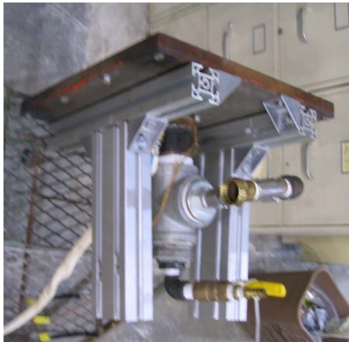
Figure 3.8: Photo of heat assembled water cooled heat flux plate
